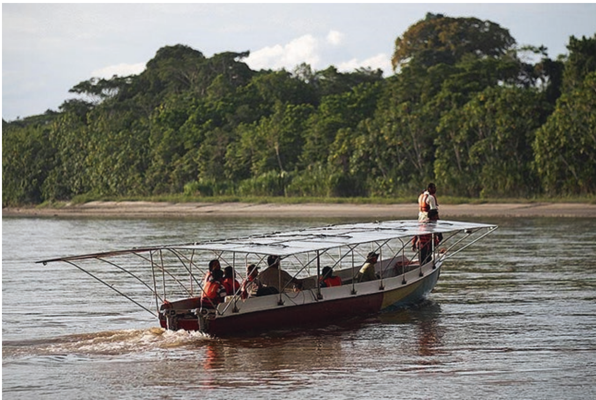
Fig. 2 Tapiatpia, the first solar canoe in the Ecuadorian Amazon. (Source: Kara Solar project photo, 2017)
