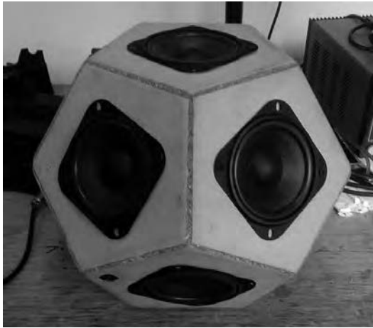
Figure 2. Final prototype of the dodecahedron speaker
