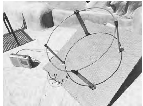
Figure 1: DIY Decametric antenna for SW news broadcast reception (Chandra, 2014)
