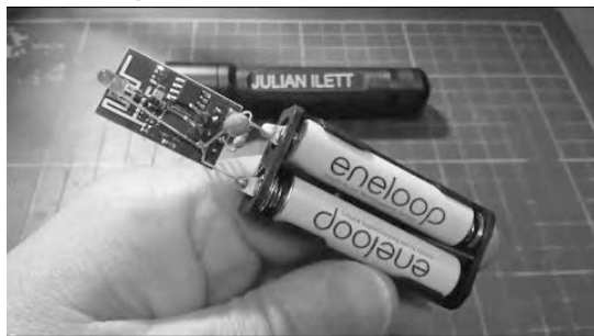
Figure 1. Recreation of the demonstration by Ilett (2015) in his project: “Web Enabled LED - WiFi Internet-of-Things IoT” Using the LUA programming language, he was able to control from a web page, electronic components connected directly to ESP8266 low power low cost module.
