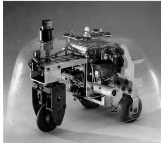
Figure 2. Grey Walter's Tortoise Elsie . Photo by Eric Long of the second generation Grey Walter turtle in the collection of the Smithsonian Institution
