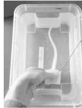
Figure 7. Physical coupling between a silicone appendix (cast onto a servo motor) and its containing medium (water). The arm produces fluid motion with gradual biomorphic bending when submerged in water but flaps clumsily around when in the air. Video: https://youtu.be/ifLChDLxdjE . ©Jonas Jørgensen
