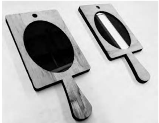
Figure 3. The idMirror device consists of a wooden case and a half mirror. A tablet computer is inserted into the case
